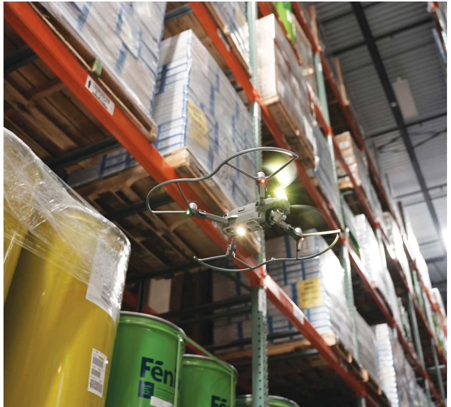
Autonomous drones are visually striking, but much of their value lies in the accurate view of current inventory they provide, which can be leveraged to update WMS.
